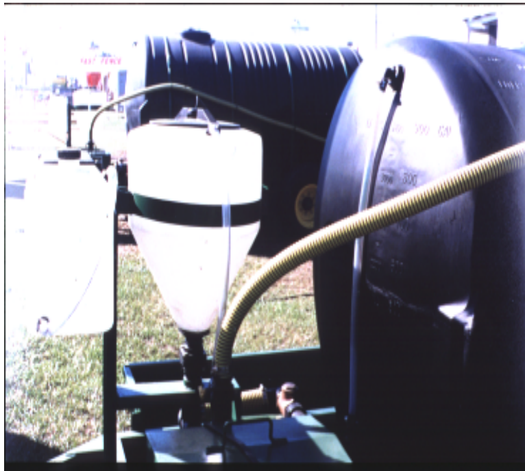
Figure 2. Nurse tank with pump, chemical inductor tank and emergency fresh water tank.
